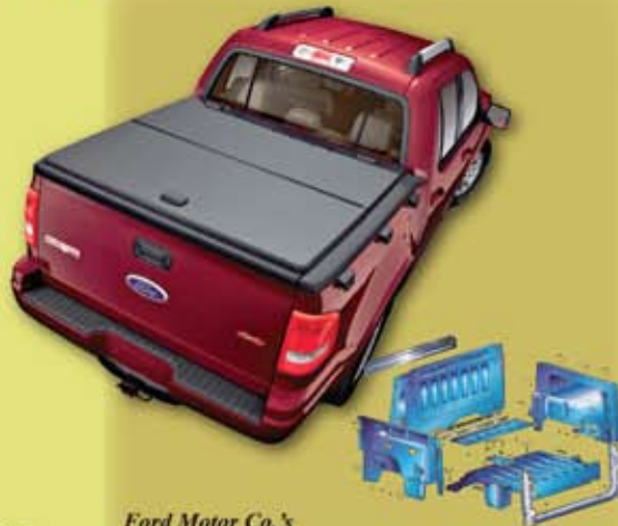
Ford Motor Co.'s re-designed SMC composite box on the 2007 Sport Trac went through some tough tests to validate the material's durability. The seven-piece box, molded by Continental Structural Plastics (formerly ThyssenKrupp Budd) uses Owens Corning glass technology.
