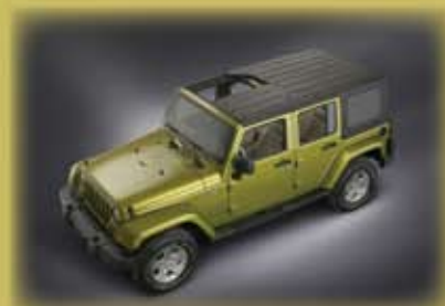
The 2007 Jeep Wrangler sports a "Freedom Top" on the two- and four-door models. The roof is molded from SMC and is comprised of three removable panels.
