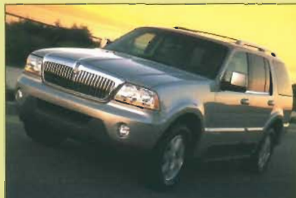
Lincoln Aviator - This all-new sports utility vehicle has sheet molded composite (SMC) front fenders and a composite grille opening reinforcement.
