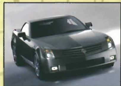
The hood, door surrounds, doors, rear quarter panels and decklid and roof combination are made of SMC on Cadillac's XLR.
