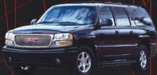
GMC Yukon Denali switches in 2001 to composite "steps," or running boards molded by Meridian Automotive Systems.
