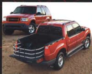
The Ford Explorer Sport Trac features the industry's first SMC cargo box – with an integrated liner, and side panels molded by Budd Plastics – made with Owens Corning's proprietary pre-form process. The ACA says the box meets 10-year, 150,000-mile durability tests. Coming soon: The Ford Super Crew Cab with four full-size doors and a composite box.
