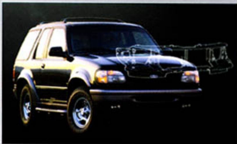
The GOR of the Ford Explorer (above) now is SMC. Prowler's SMC windshield frame (below) surrounds the glass and is a structurally loaded assembly.
